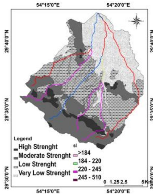
Fig. 2. Geological strength levels and distribution of SL index anomalies for Shahriary basin
