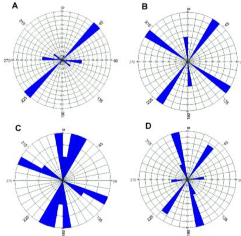
Fig. 9. Direction and frequency of fractures in the Shahriary catchment
