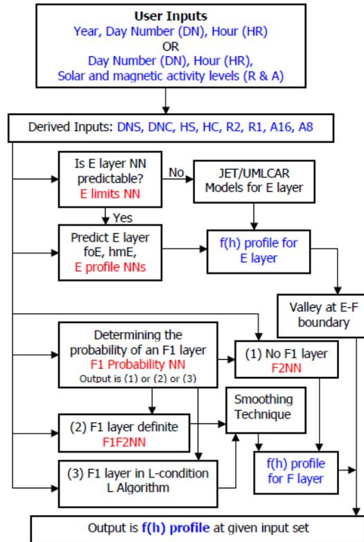
Fig. 1. A flow diagram illustrating the process followed by SABIM in determining the predicted profile (McKinnell, 2002)
